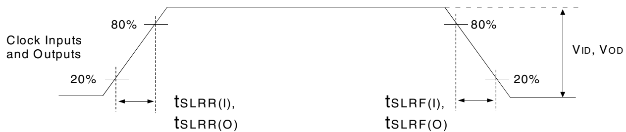
Figure 8. Input and Output Slew Rates
