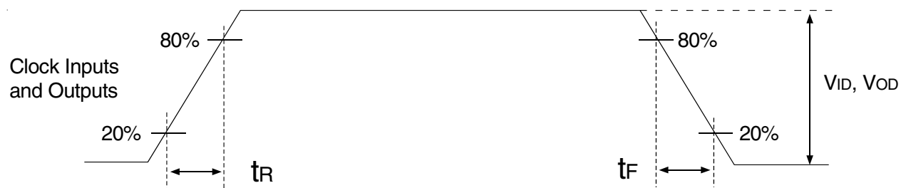
Figure 8. Input and Output Slew Rates
