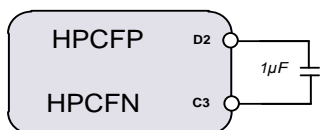
Figure 39. Charge pump flying capacitor
