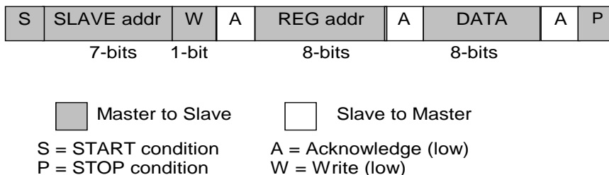
Figure 34: I 2 C Byte Write (SDA line)
