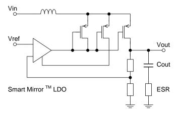
Figure 16: Smart Mirror Voltage Regulator
