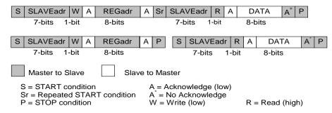
Figure 11: Examples of Byte Read Operations
