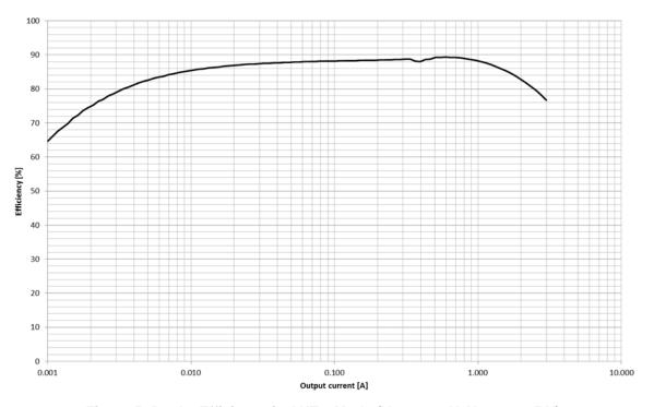
Figure 5: Buck1 Efficiency in AUTO Mode ( $V_{IN} = 3.60 \text{ V}$ ,  $V_{OUT} = 1.15 \text{ V}$ )
