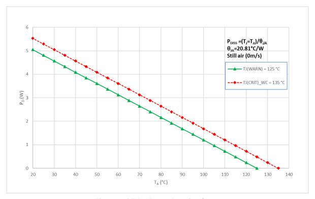
Figure 3: QFN40 Power Derating Curve
