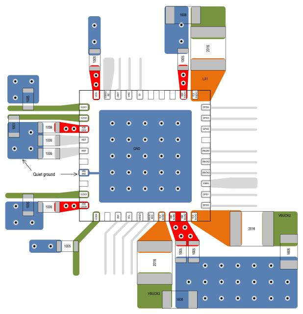
Figure 20: PCB Layout for DA9061-A
