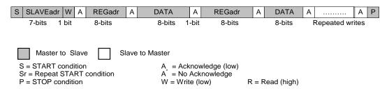
Figure 14: 2-Wire Repeated Write
