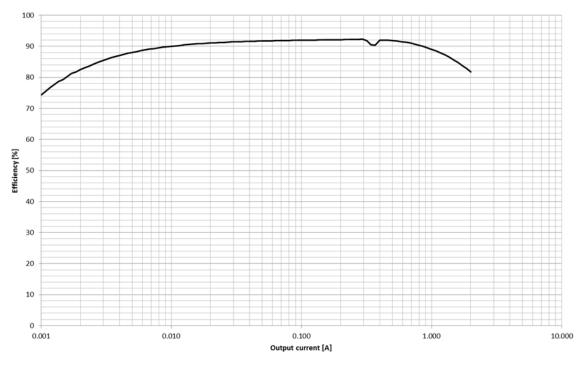
Figure 6: Buck2 Efficiency in AUTO Mode ( $V_{IN} = 3.60 \text{ V}, V_{OUT} = 1.80 \text{ V}$ )
