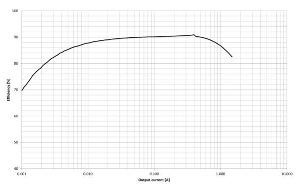
Figure 8: Buck3 Efficiency in AUTO Mode ( $V_{IN} = 3.60 \text{ V}$ ,  $V_{OUT} = 1.35 \text{ V}$ )
