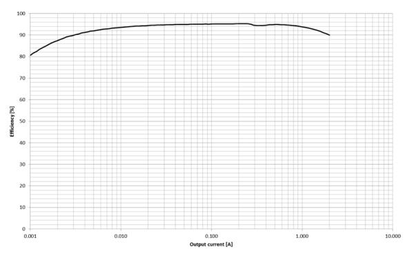
Figure 7: Buck2 Efficiency in AUTO Mode (V<sub>IN</sub> = 5.00 V, V<sub>OUT</sub> = 3.34 V)
