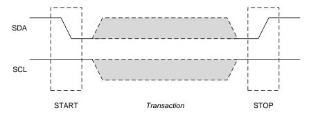
Figure 9: Timing of the START and STOP Conditions
