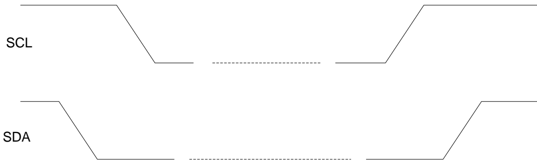
Figure 16: I 2 C START and STOP Condition Timing
