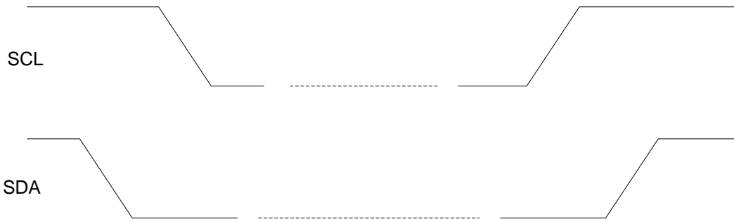
Figure 21: I 2 C START and STOP Condition Timing
