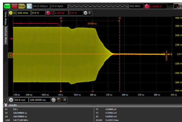
Figure 16. Switching Time Insertion Loss to Isolation State
