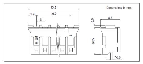
Figure 8. Receptacle Drawing
