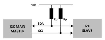
Figure 3. I<sup>2</sup>C Master-Slave Configuration
