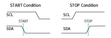
Figure 4. START and STOP Condition Waveform
