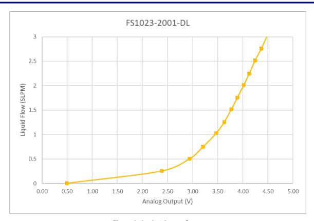
Figure 2. Analog Output Curve
