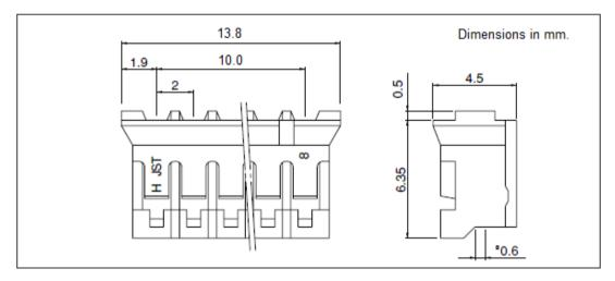
Figure 8. Receptacle Drawing
