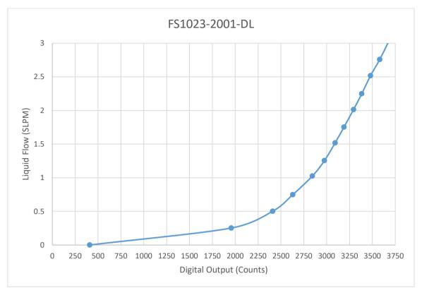
Figure 1. Digital Output Curve
