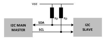
Figure 4. I2C Master-Slave Configuration
