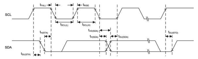
Figure 1. I2C Timing Diagram
