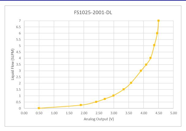
Figure 3. Analog Output Curve
