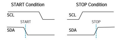
Figure 5. START and STOP Condition Waveform
