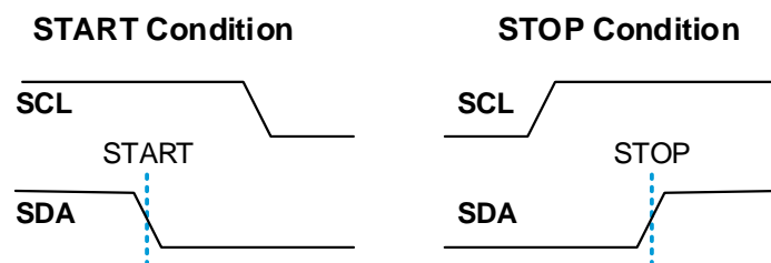
Figure 4. START and STOP Condition Waveform
