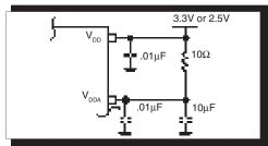
FIGURE 1. POWER SUPPLY FILTERING
