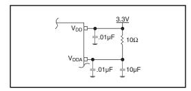
Figure 1. Power Supply Filtering
