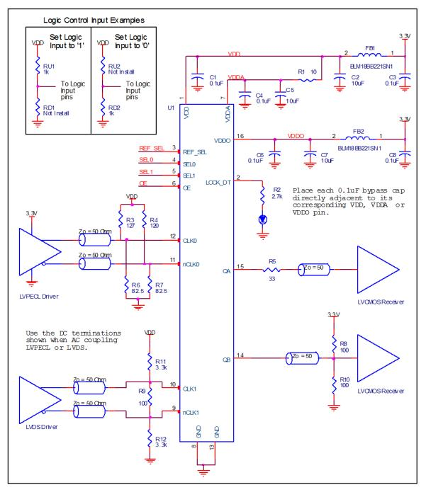
Figure 4. ICS840272I Schematic Example
