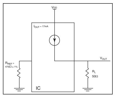
Figure 4. HCSL Driver Circuit and Termination
