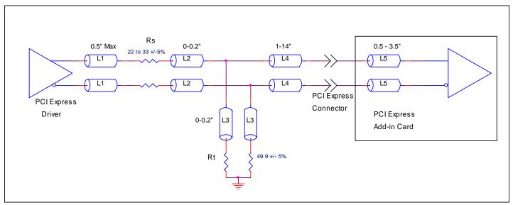
Figure 2A. Recommended Source Termination (where the driver and receiver will be on separate PCBs)
