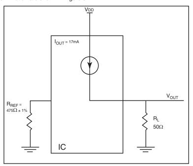
FIGURE 8. HCSL DRIVER CIRCUIT AND TERMINATION
