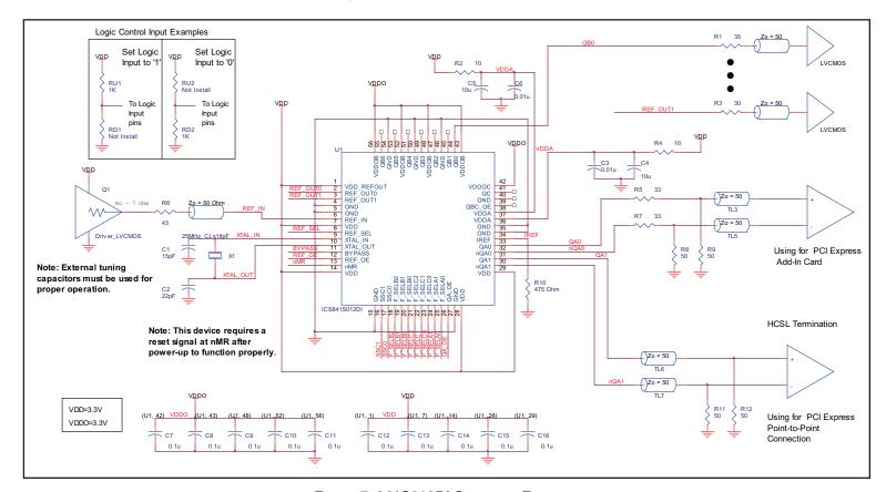
FIGURE 7. 841S012DI SCHEMATIC EXAMPLE
