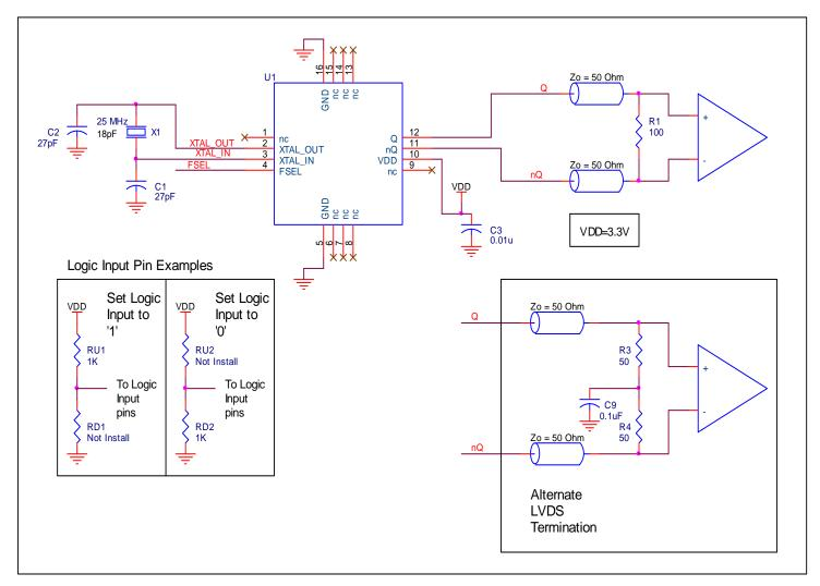
Figure 4. ICS844201I-45 Schematic Example
