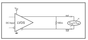
**Differential Output Voltage Setup**
