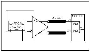
3.3V LVDS Output Load AC Test Circuit
