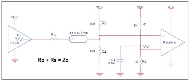
FIGURE 2. SINGLE ENDED SIGNAL DRIVING DIFFERENTIAL INPUT
