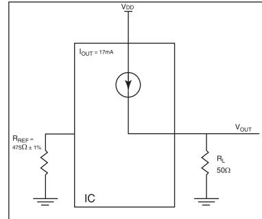
HCSL output driver circuit and termination are shown in Figure 5.
