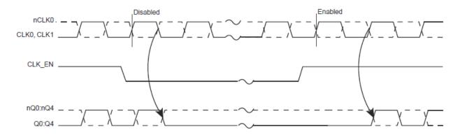
FIGURE 1. CLK\_EN TIMING DIAGRAM
