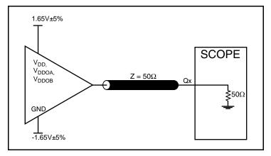
3.3V Output Load Test Circuit
