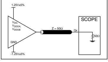
2.5V Output Load Test Circuit
