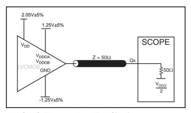
3.3V Core/2.5V Output Load Test Circuit
