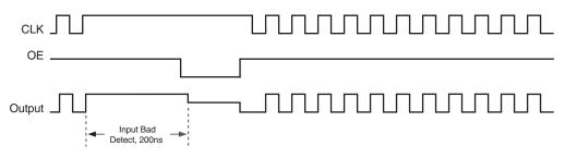
Figure 1F. OEx with Bad Input Timing Diagram
