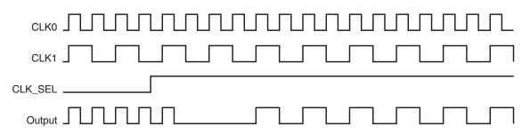
Figure 1A. CLK\_SEL Timing Diagram
