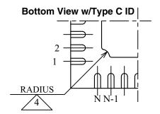
There are 2 methods of indicating pin 1 corner at the back of the VFQFN package:
