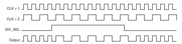
Figure 1B. DIV\_SELx Timing Diagram
