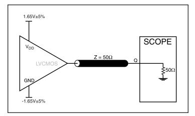
3.3V LVCMOS Output Load Test Circuit
