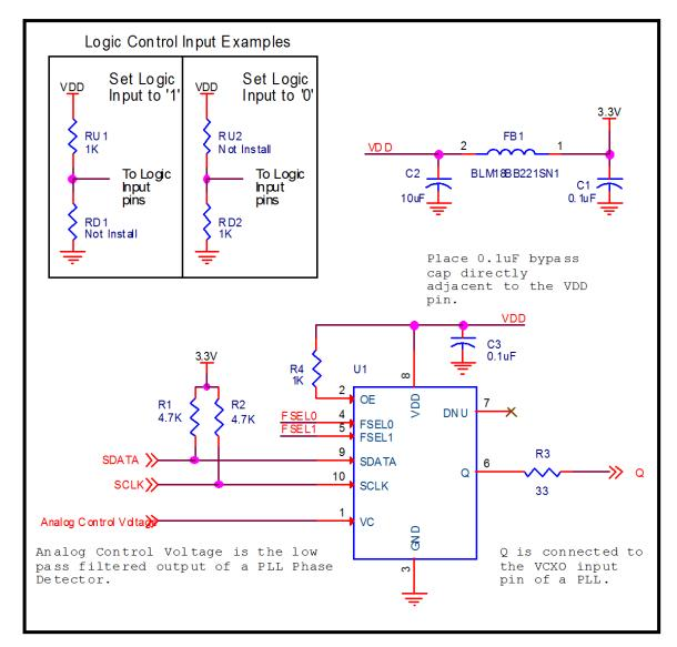
Figure 1. IDT8N0QV01 Schematic Example
