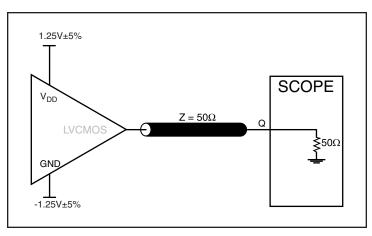
2.5V LVCMOS Output Load Test Circuit
