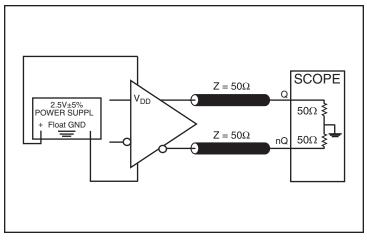
3.3V LVDS Output Load AC Test Circuit
