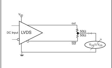
**Differential Output Voltage Setup**
