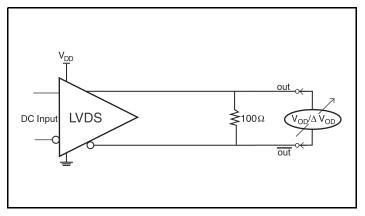
**Differential Output Voltage Setup**
