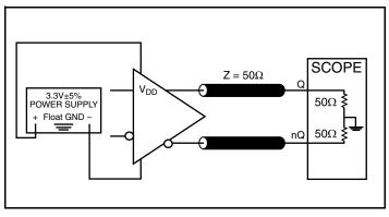
3.3V LVDS Output Load Test Circuit
