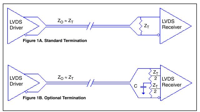
Figure 1. Typical LVDS Driver Termination
