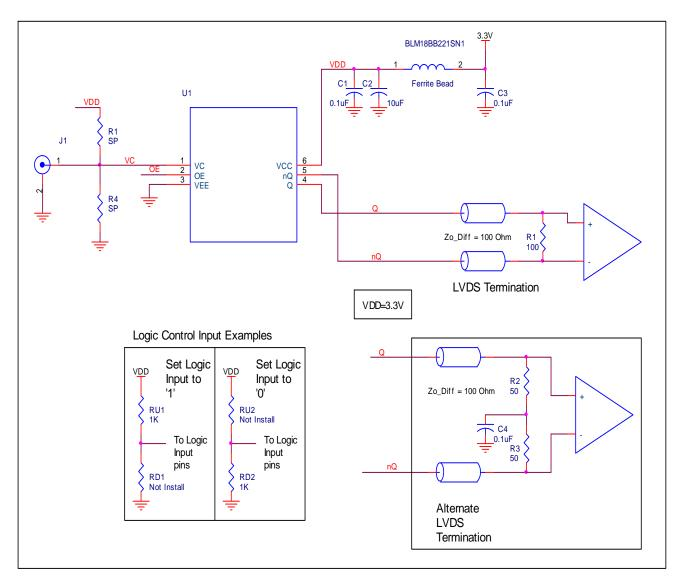
Figure 2. IDT8N4SV75 Schematic Example
