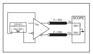
2.5V LVDS Output Load AC Test Circuit
