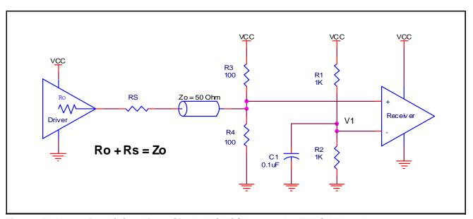
Figure 1B. Alternative DC Coupling a Single LVCMOS Input to the IDT8SLVP2106I
