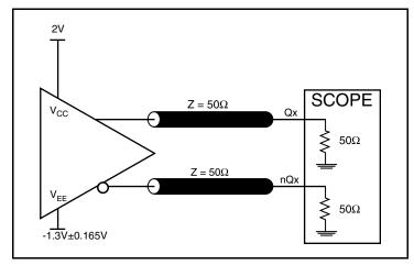
3.3V LVPECL Output Load Test Circuit
