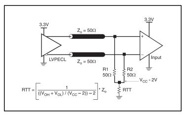
Figure 5A. 3.3V LVPECL Output Termination
