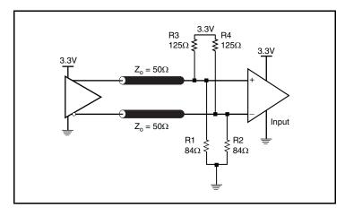
Figure 5B. 3.3V LVPECL Output Termination
