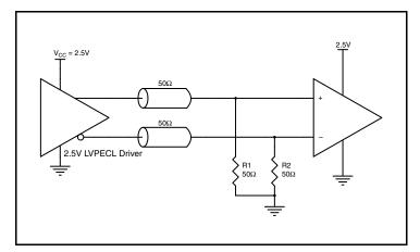
Figure 6C. 2.5V LVPECL Driver Termination Example
