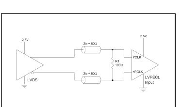
Figure 3C. PCLK/nPCLK Input Driven by a 2.5V LVDS Driver
