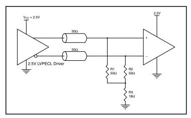
Figure 6B. 2.5V LVPECL Driver Termination Example
