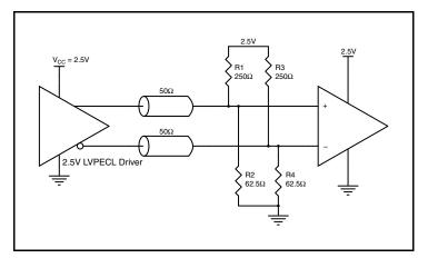
Figure 6A. 2.5V LVPECL Driver Termination Example
