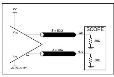
2.5V LVPECL Output Load Test Circuit
