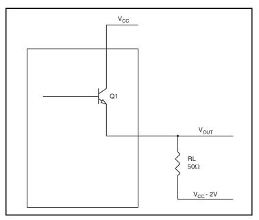
Figure 7. LVPECL Driver Circuit and Termination
