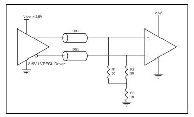
Figure 7B. 2.5V LVPECL Driver Termination Example
