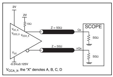
2.5V LVPECL Output Load Test Circuit
