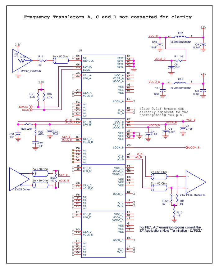
Figure 8. IDT8T49N445I Schematic Example
