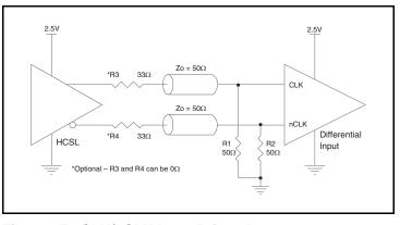
Figure 5E. CLK/nCLK Input Driven by a 2.5V HCSL Driver
