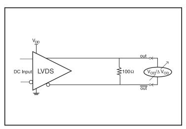
**Differential Output Voltage Setup**
