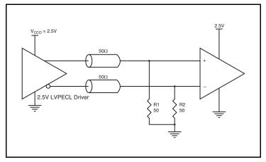
Figure 7C. 2.5V LVPECL Driver Termination Example
