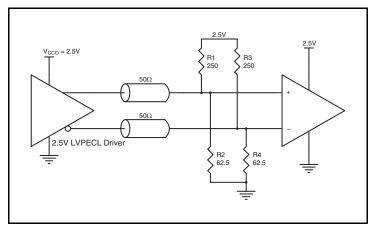
Figure 7A. 2.5V LVPECL Driver Termination Example
