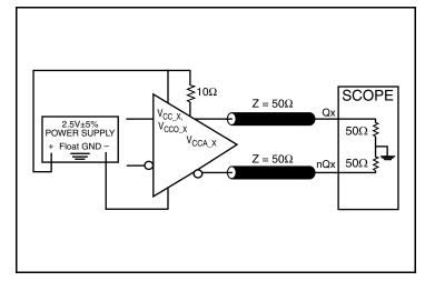
2.5V LVDS Output Load Test Circuit
