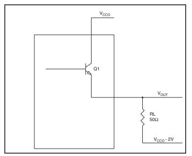
Figure 9. LVPECL Driver Circuit and Termination
