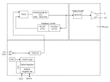
Figure 2. High Bandwidth Frequency Translator Mode Block Diagram
