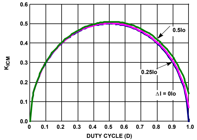
FIGURE 11. INPUT-CAPACITOR CURRENT MULTIPLIER FOR SINGLE-PHASE BUCK CONVERTER
