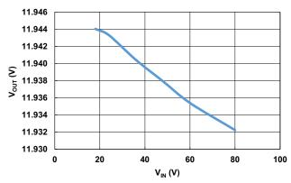
Figure 21. CCM Line Regulation at 20A Load +25°C
