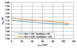
Figure 8. V<sub>DD</sub> Load Regulation at 12V Input
