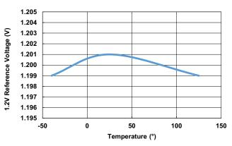
Figure 15. 1.2V Reference Voltage vs Temperature
