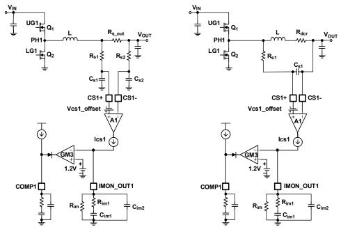
A. I<sub>OUT</sub> Average Current Loop with Shunt Sense
