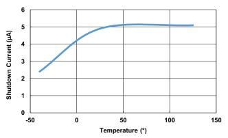
Figure 6. Shutdown Current vs Temperature
