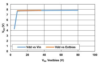
Figure 9. V<sub>DD</sub> Line Regulation at 20mA Load
