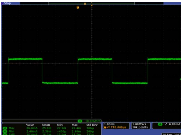
FIGURE 13. I_{LED} AT 50% PWM DIMMING
