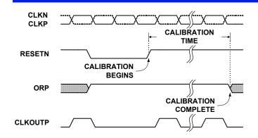
FIGURE 25. CALIBRATION TIMING
