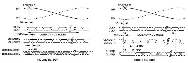
FIGURE 4. LVDS TIMING DIAGRAMS (See "Digital Outputs" on page 21)
