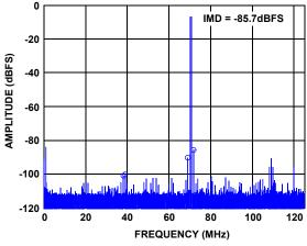
FIGURE 22. TWO-TONE SPECTRUM AT 70MHz
