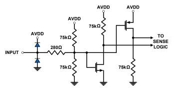
FIGURE 46. TRI-LEVEL DIGITAL INPUTS
