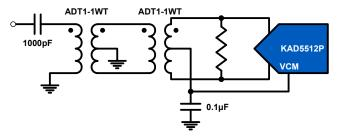
FIGURE 29. TRANSFORMER INPUT FOR GENERAL PURPOSE APPLICATIONS
