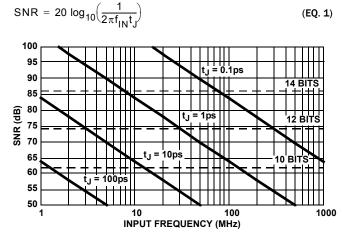
FIGURE 33. SNR vs CLOCK JITTER
