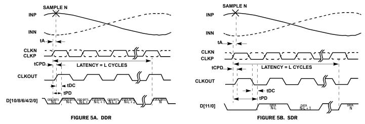
FIGURE 5. CMOS TIMING DIAGRAM (See "Digital Outputs" on page 21)
