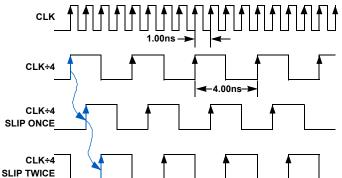
FIGURE 42. PHASE SLIP: CLK $\div$ 4 MODE,  $f_{CLOCK} = 1000MHz$
