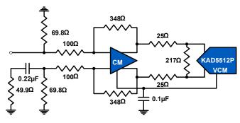
FIGURE 31. DIFFERENTIAL AMPLIFIER INPUT
