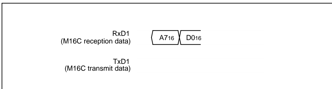
Figure 1.29.28. Timing for erasing all unlocked blocks
