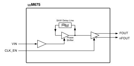
Figure 2: Block Diagram
