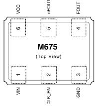
Figure 1: Pin Assignment
