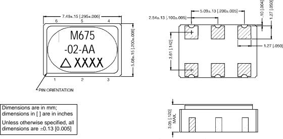
Figure 5: Device Package - 5 x 7.5mm SMT (Surface Mount) Package
