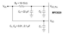
Figure 4. V<sub>CC PLL</sub> Power Supply Filter
