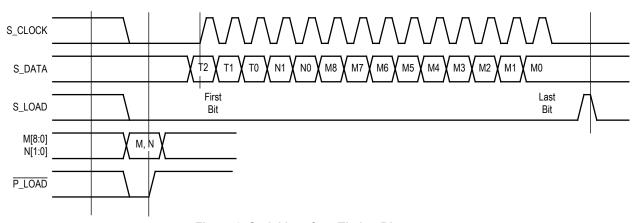
Figure 3. Serial Interface Timing Diagram
