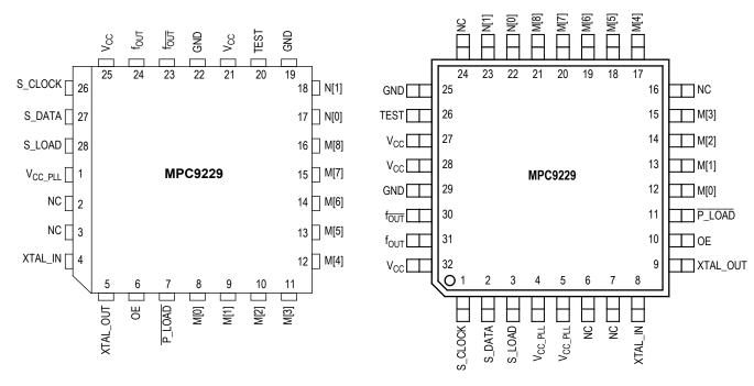
Figure 2. MPC9229 28-Lead PLCC Pinout (Top View)
