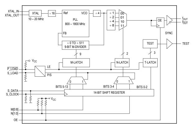
Figure 1. MPC9229 Logic Diagram
