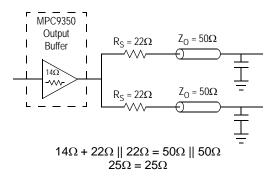
Figure 6. Optimized Dual Line Termination
