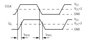
Figure 8. Propagation Delay (t<sub>PD</sub>) Test Reference
