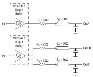
Figure 4. Single versus Dual Transmission Lines
