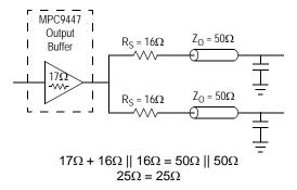
Figure 6. Optimized Dual Line Termination
