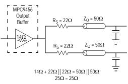
Figure 5. Optimized Dual Line Termination
