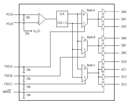
Figure 1. MPC9456 Logic Diagram
