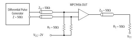
Figure 6. PCLK MPC9456 AC Test Reference for V<sub>CC</sub> = 3.3 V and V<sub>CC</sub> = 2.5 V
