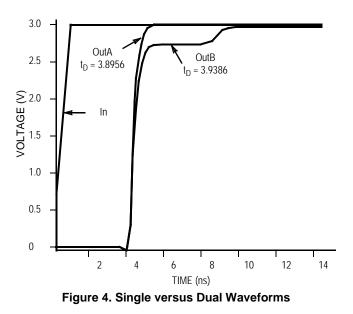
Since this step is well above the threshold region it will not cause any false clock triggering, however designers may be uncomfortable with unwanted reflections on the line. To better match the impedances when driving multiple lines the situation in Figure 5 should be used. In this case the series terminating resistors are reduced such that when the parallel combination is added to the output buffer impedance the line impedance is perfectly matched.
