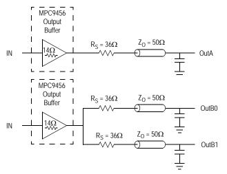
Figure 3. Single versus Dual Transmission Lines
