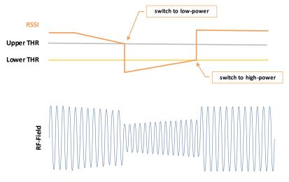
Figure 7: Dynamic Digital Power Control (DDPC)
