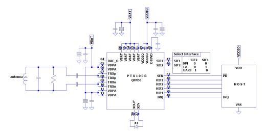
Figure 10: Exemplary Reference Schematic
