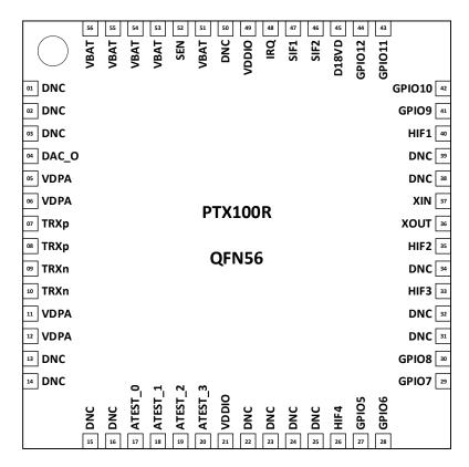
Figure 2: Pin Diagram
