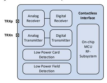
Figure 6: Contactless Interface
