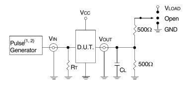
Test Circuits for All Outputs
