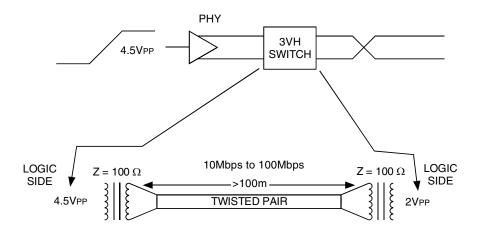
Fast Ethernet Data Switching (LAN Switch)
