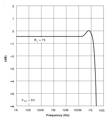
Insertion Loss vs. Frequency
