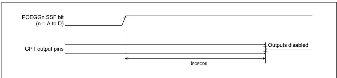
Figure 2.19 Output Disable Time for POEG in Response to the Register Setting
