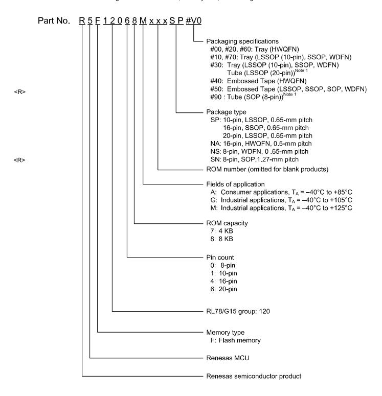
Note 1. For the 8-pin SOP, and the 20-pin LSSOP products only, the packaging specification is Tube.
