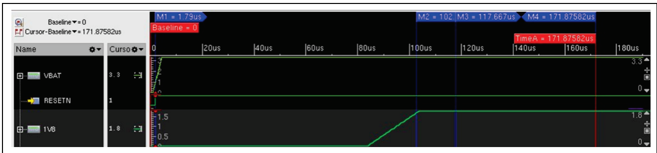
Figure 4. Timing Diagram for Power-Up Sequence
