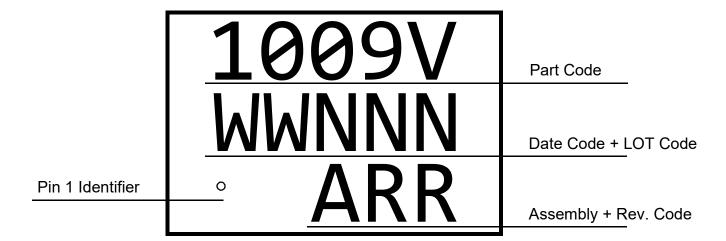
1009V - Part ID Field WW - Date Code Field<sup>1</sup> NNN - Lot Traceability Code Field<sup>1</sup> A - Assembly Site Code Field<sup>2</sup> RR - Part Revision Code Field<sup>2</sup>
