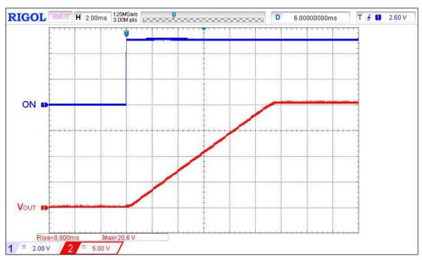
Figure 3. Typical Turn ON operation waveform for  $V_{IN}$  = 20 V,  $C_{SLEW}$  = 18 nF,  $C_{LOAD}$  = 10  $\mu$ F,  $R_{LOAD}$  = 100  $\Omega$  Typical Turn-off Waveforms
