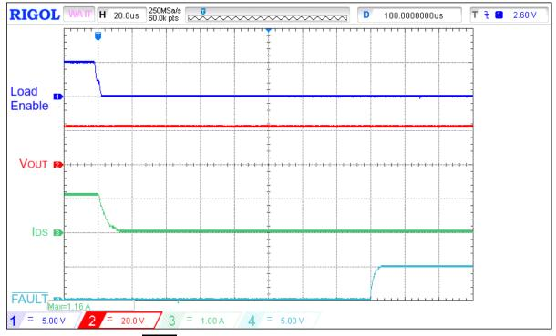
Figure 8. Typical FAULT de-assertion waveform for V<sub>IN</sub> = 20 V, C<sub>LOAD</sub> = 10  $\mu$ F, I<sub>ACL</sub> = 1 A, R<sub>SET</sub> = 91 k $\Omega$ , switch out 20  $\Omega$  load
