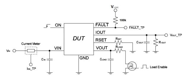
Figure 1. Test setup Application Diagram
