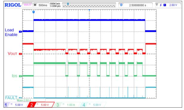
Figure 6. Typical ACL operation waveform for V<sub>IN</sub> = 4.5 V, C<sub>LOAD</sub> = 10  $\mu$ F, I<sub>ACL</sub> = 1 A, R<sub>SET</sub> = 91 k $\Omega$
