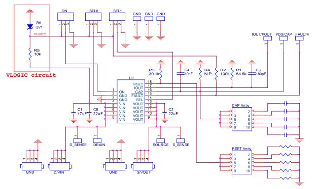
Figure 11. SLG59H1126V Evaluation Board Connection Circuit
