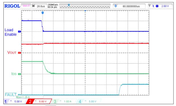
Figure 9. Typical FAULT de-assertion waveform for V<sub>IN</sub> = 4.5 V, C<sub>LOAD</sub> = 10  $\mu$ F, I<sub>ACL</sub> = 1 A, R<sub>SET</sub> = 91 k $\Omega$ , switch out 3.3  $\Omega$  load
