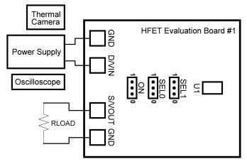
Figure 12. SLG59H1126V Evaluation Board Connection Circuit
