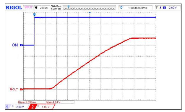
Figure 2. Typical Turn ON operation waveform for V<sub>IN</sub> = 4.5 V, C<sub>SLEW</sub> = 10 nF, C<sub>LOAD</sub> = 10  $\mu$ F, R<sub>LOAD</sub> = 100  $\Omega$
