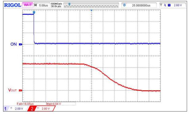
Figure 4. Typical Turn OFF operation waveform for V<sub>IN</sub> = 4.5 V, C<sub>SLEW</sub> = 10 nF, no C<sub>LOAD</sub> , R<sub>LOAD</sub> = 100  $\Omega$
