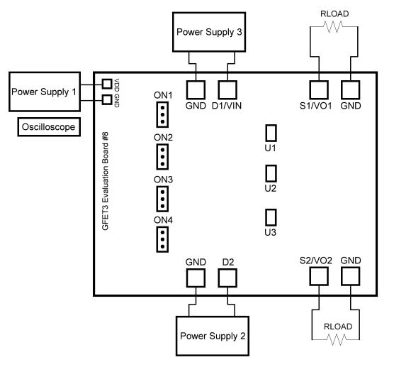
Figure 3. SLG59M1527V Evaluation Board Connection Circuit
