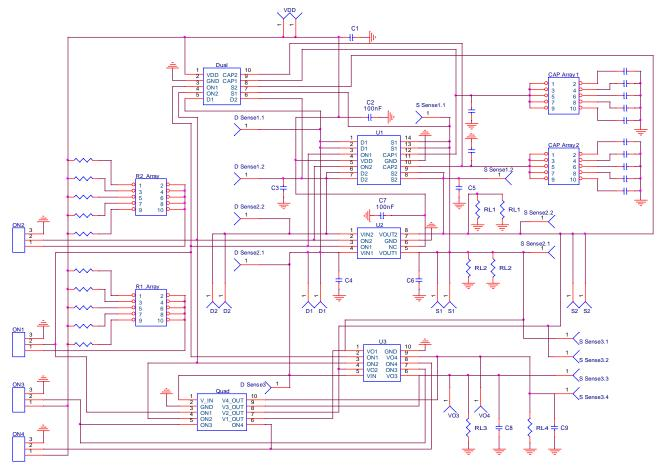
Figure 2. SLG59M1527V Evaluation Board Connection Circuit
