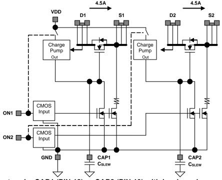
Do not probe CAP1 (PIN 12) or CAP2 (PIN 10) with low impedance probe.
