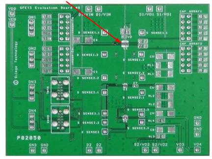
Figure 1. SLG59M1527V Evaluation Board
