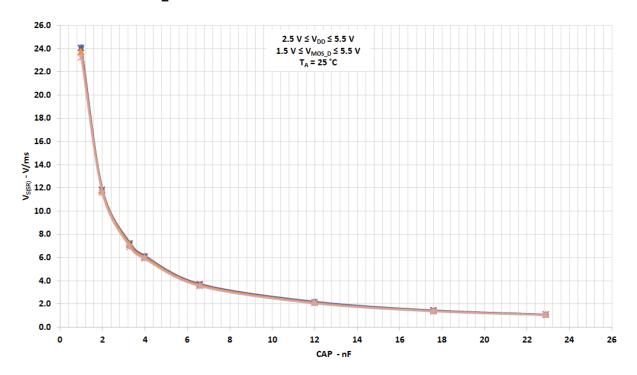
$\rm T_{Total\_ON}$  vs. CAP,  $\rm V_{MOS\_D},$  and  $\rm V_{DD}$
