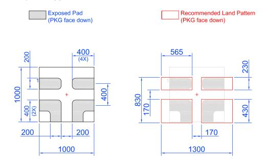
Note: All dimensions shown in micrometers (µm)
