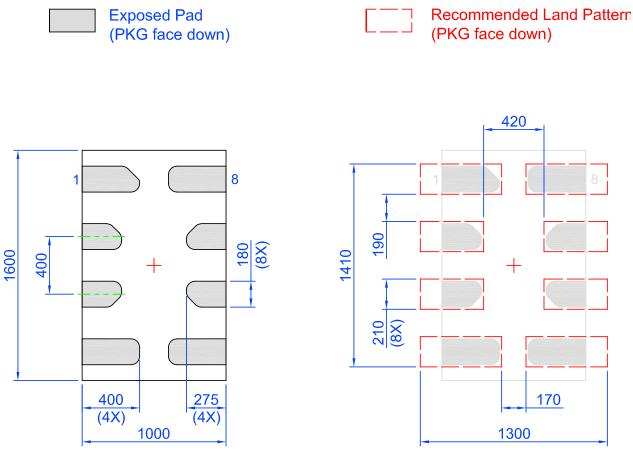
Note: All dimensions shown in micrometers (µm)
