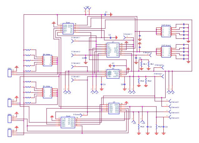
Figure 2. SLG59M1641V Evaluation Board Connection Circuit
