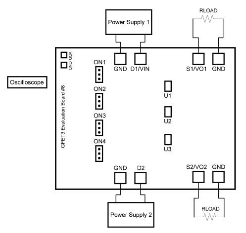
Figure 3. SLG59M1641V Evaluation Board Connection Circuit
