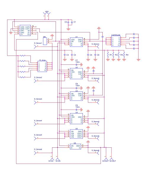
Figure 2. SLG59M301V Evaluation Board Connection Circuit.
