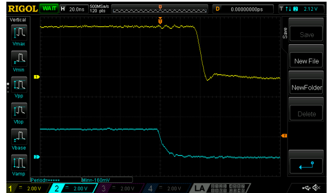
6. Transient from High to Low (PIN# 18 (SPI1_DIN) => PIN# 4 (RZ_RSPI1_MISO))
