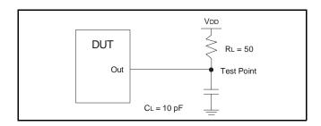
Load Circuit: High-to-Low Slew-Rate Adjustment
