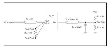
**Simulation Load Circuit**
